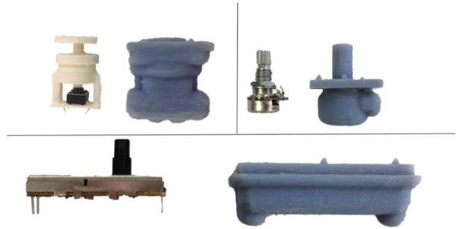
Figure 10 A widget set together with printed blanks used in sculpting. The widgets are a button on the top left, a knob on the top right and a slider on bottom. The button includes a complex mounting bracket printed in white and a moving plunger.
