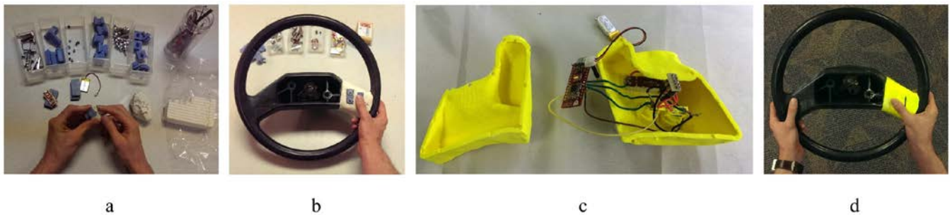
Figure 2 Sculpting around printed blanks that represent widgets to make an interactive physical device.
